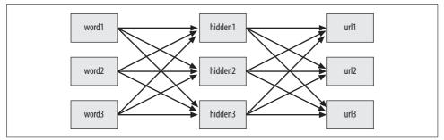
Figure 4-4. Design of a click-tracking neural network
