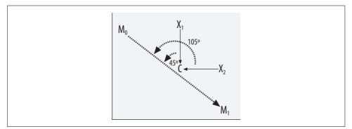
Figure 9-6. Using dot-products to determine distance
