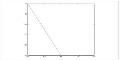
Figure 8-4. Subtraction weight function
