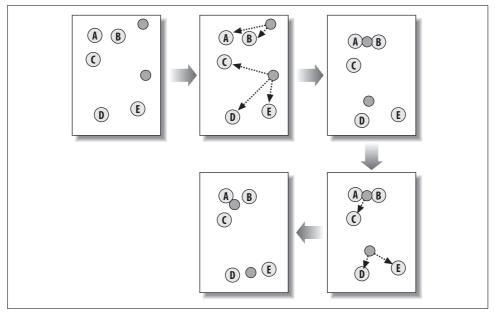
Figure 12-14. Process of K-means clustering
